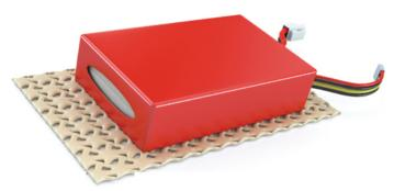
Place a piece of rubber tool-drawer liner material under your battery pack before you secure the pack with a Velcro strap, and the liner will prevent it from slipping out.
