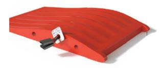
Here's an easy way to prevent those aileron and flap Y-harness leads from slipping inside the fuselage or wing. When the leads are disconnected from the wings, use the little plastic tabs that keep plastic bread bags closed and clip them over the end of the servo leads to prevent them from falling back into the fuselage. Everyone has at least a couple of these things lying around, so you might as well put them to good use.
